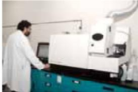
The majority of elemental analysis is performed by ICP and ICP/MS simultaneous instrumentation. Our Trace ICP's and ICP/MS allow very sensitive MDL's to be achieved. They are used for the determination of dissolved, suspended, or total elements in industrial waste water, drinking, surface or ground water. This technique can analyze up to 30 elements in a single analysis. Analytical tests routinely performed by ICP include:
